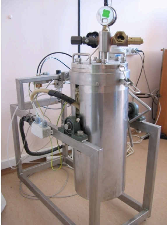
Figure 8. Custom made pulping stainless 2 L autoclave
