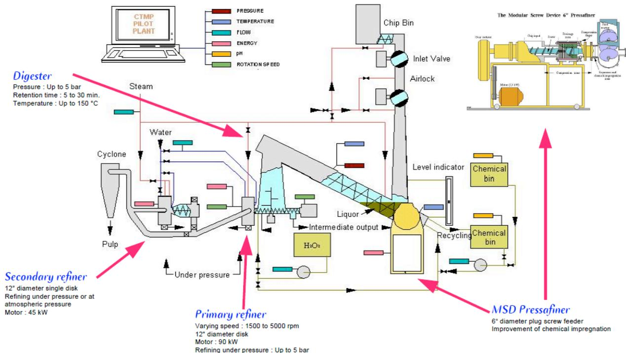
Figure 13. **Large scale thermomechanical pulping pilot at InTechFibres facilities.**
