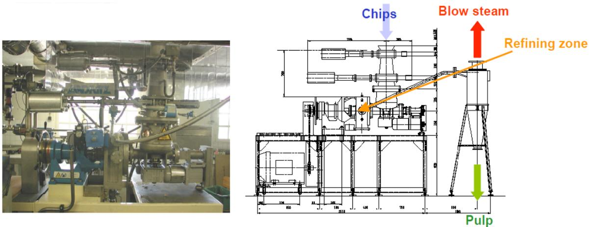
Figure 12. Small scale thermomechanical pulping pilot at InTechFibres facilities.
