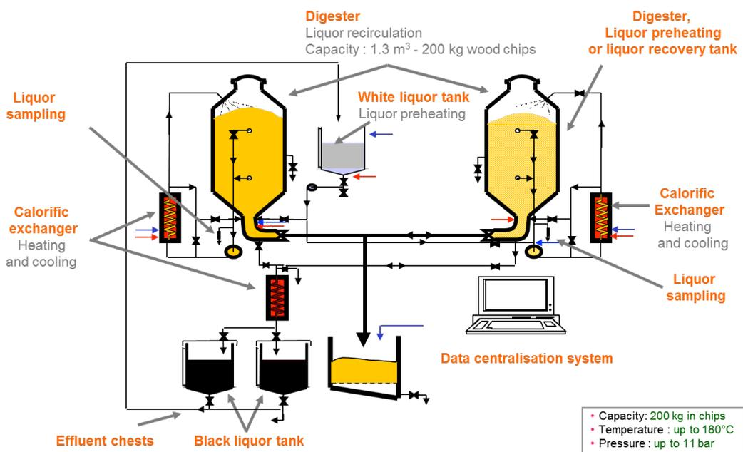
Figure 10. Cooking pilot plant at InTechFibres facilities.
